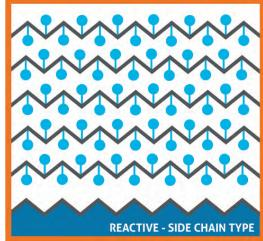
**Gray** lines represent the polymer chains of the material to which an FR is applied.
