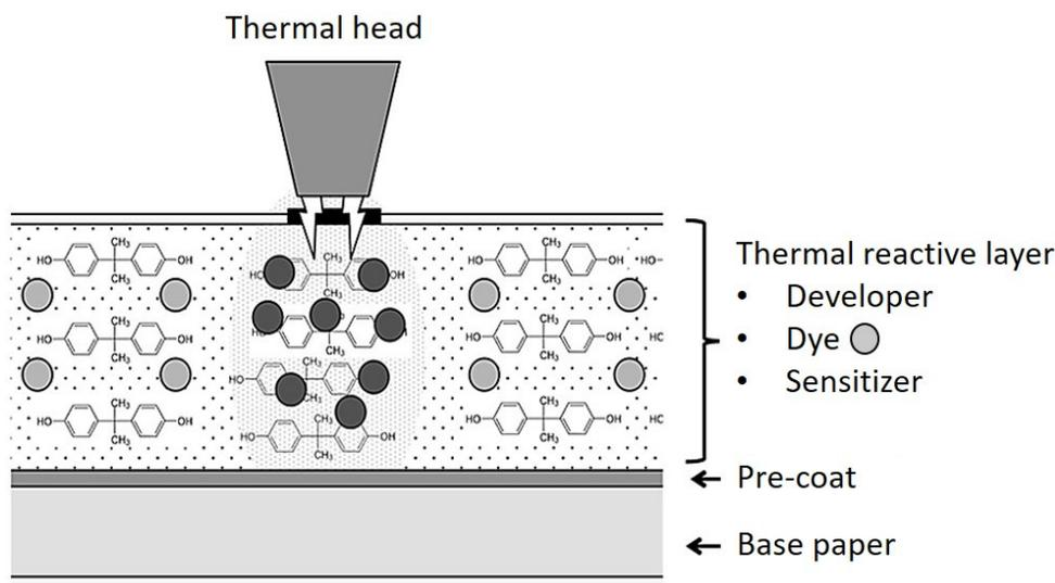
**Figure 1:** Diagram of thermal paper. (Hormann *et al.* 2014)
