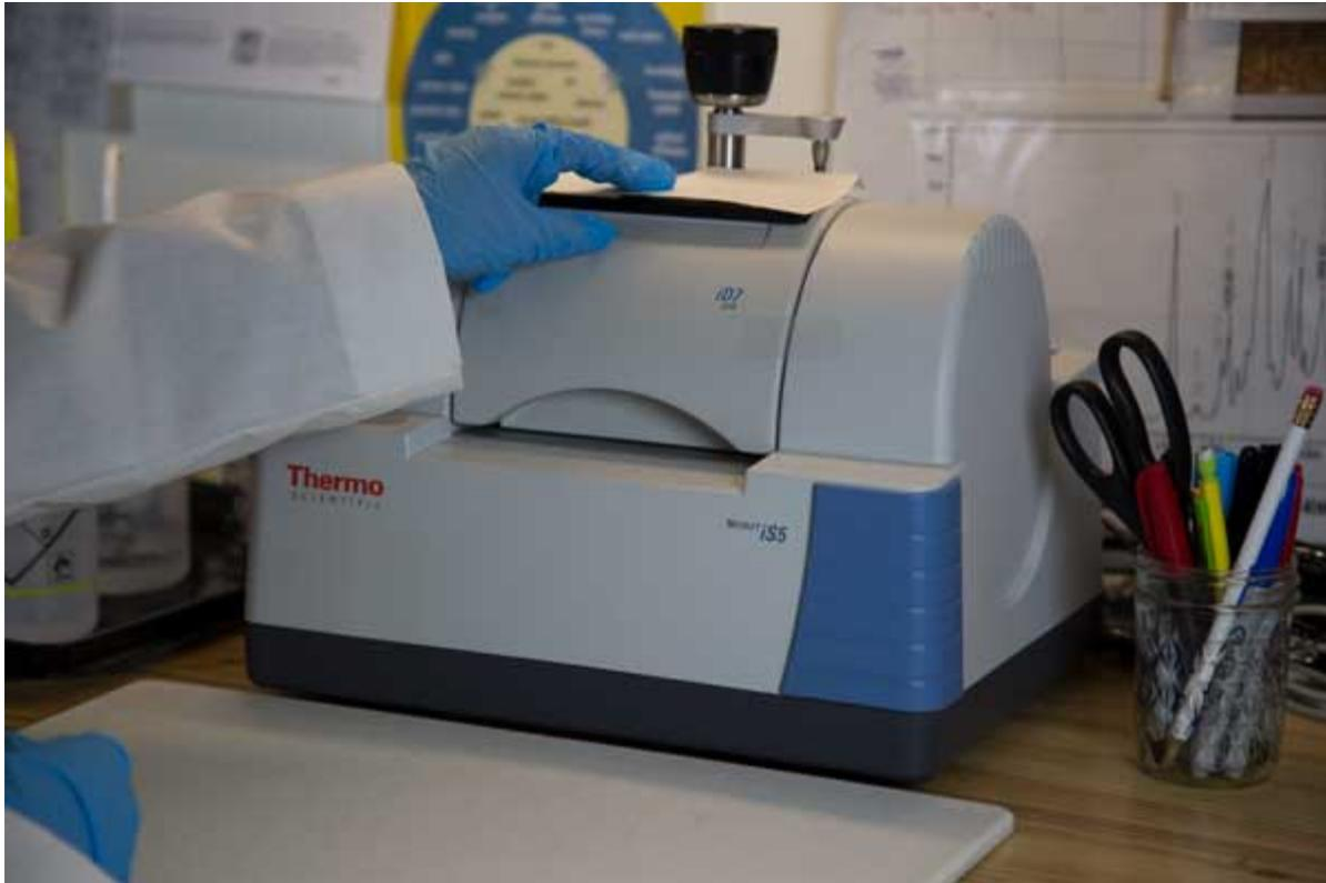
**Figure 3.** Receipt undergoing ATR-FTIR testing.
